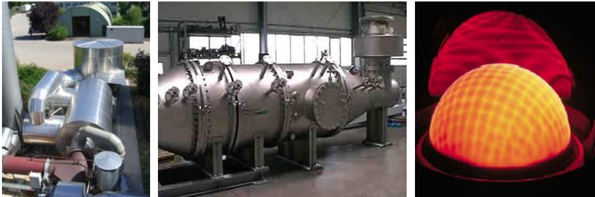
Figure 4: Pictures of two systems for the catalytic oxidation of combustible gases, view of the catalytic Matrix burner in operation (Source: Dürr Clean Technology Systems AG, R.Scheuchl GmbH, Viessmann GmbH & Co. KG)
