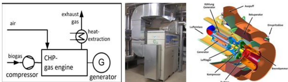
Figure 2: Flow sheet of a gas turbine for the combined production of electricity and heat; illustration of a Capstone ® microgas turbine system and sectional drawing of a Capstone ® microgas turbine
